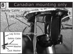
For Canadian installation in both flush and downrod mode the safety cable must be installed into the house structure beams using the 3" lag screws provided. Make sure that when the safety cable is fully extended the leadwires are longer than the cable and no stress is placed on the leadwires.
